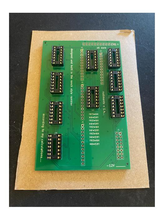
I use the cardboard to help flip the board over with the IC sockets placed. Solder away! but be careful of those SMDs! The picture has a pinpoint tip but I actually grew to prefer the T-18 D16 tip, as the ground connections can suck up a lot of heat!
