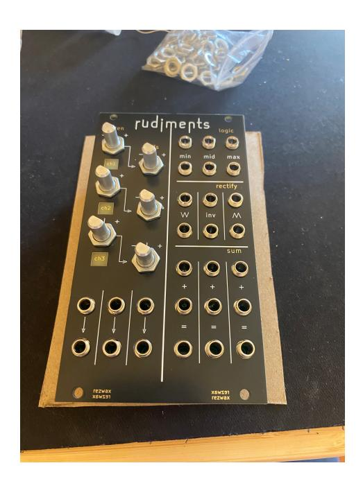
You might have to finnagle my wonky LEDs to be touching the front panel and in position, but DO SO CAREFULLY. I have broken traces from scratching the panel with needlenose pliers. It should be green on top directly below the window, and red below just outside of the window.
