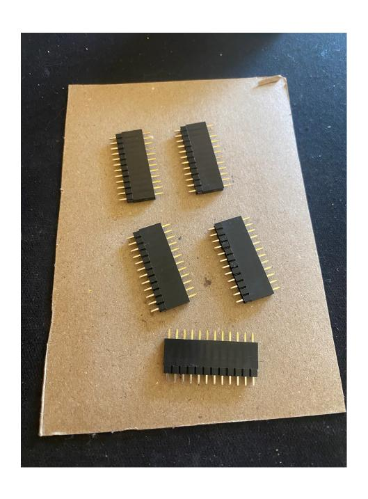
This part is a little annoying, but you have to kind of balance these upright and slide the interface board into place on top. I usually start with the top horizontal header and try to angle it down onto the vertical bottom 4.
