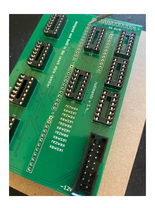
Now separate your boards, and get ready for placing all those dang jacks and pots. I actually find the opposite of this image to be the better male/female configuration, as soldering all those jacks and pots with metal pins to avoid instead of the plastic header is much less strenuous.
