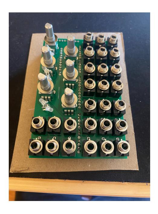
Place the panel and screw the pots in place to make anbother sandwich and keep the jacks in place while soldering. If youre using helping hands place a thin cardboard buffer around the part of the faceplate to prevent any unsightly claw tooth marks.
