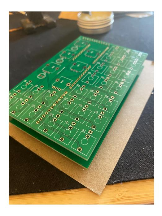
I usually try to solder the ground pins on both sides so that I wont have to worry about it falling apart if I move it. But it is a delicate balancing act! The ground pins are only in the middle row as depicted to the left.
