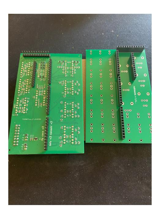
Place and solder those jacks and LEDs, if youre using my LEDs the cathode (flat side of the circle on the PCB) is marked green. Because the Red is "brighter" than the Green at the same voltage, I found that placing the green directly under the window and the red just outside of the window produced the most even results. Plus it kind of creates a movement that I find pleasing, instead of the two colors coming from the same location.
